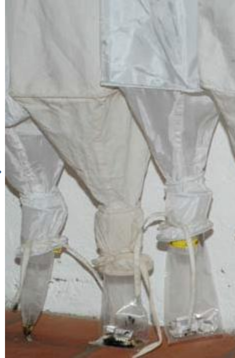
Extraction of ants from the leaf litter with a Winkler for 48h
